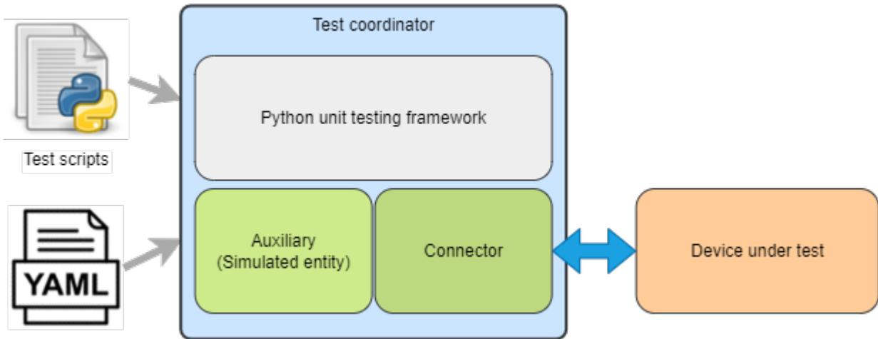
The *pykiso* ITF is built in a modular and configurable way with abstractions for both, entities (e.g. simulated counterpart for the device under test) and communication (e.g. UART or TCP/IP).
